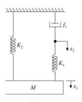
3. Determine the transfer function of the given System using block diagram reduction technique or Manson's gain formula . (BT-2)
